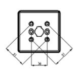
For its installation, fix the MCP box to the wall by means of 2 screws using the fastening openings provided for this purpose, introducing the connection cables through the opening located in the central part of the box. Before installing the MCP unit it has to be coded as indicated on the last page.
